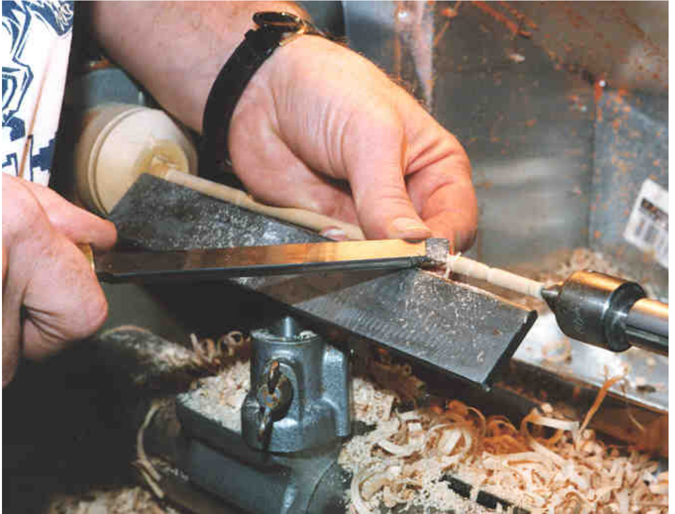
After turning the shaft is sanded smooth:
