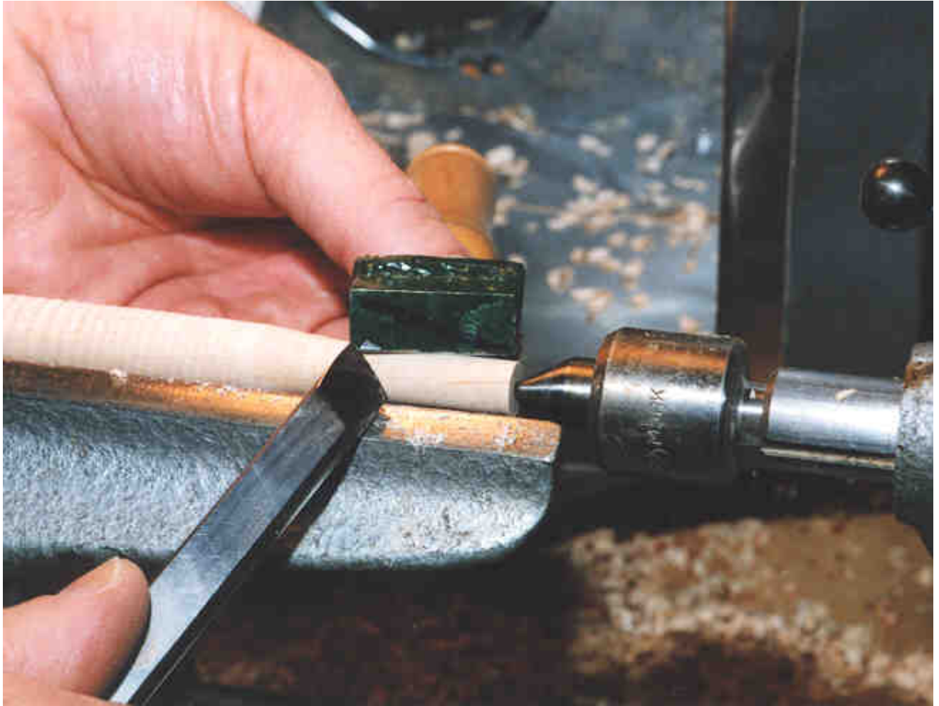
After the taper is turned I turn decorative beads and a cove on the end of the shaft:
