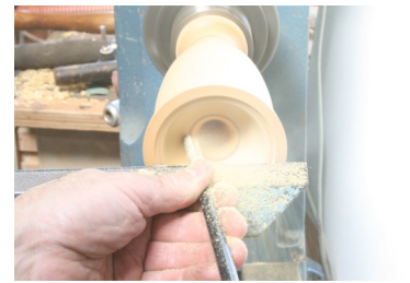
Turn out inside to 6mm wall thickness
