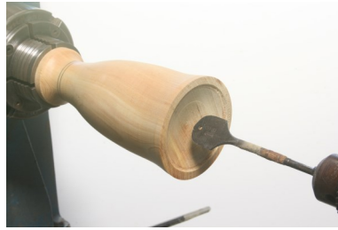
Drill with round end speed bore drill
