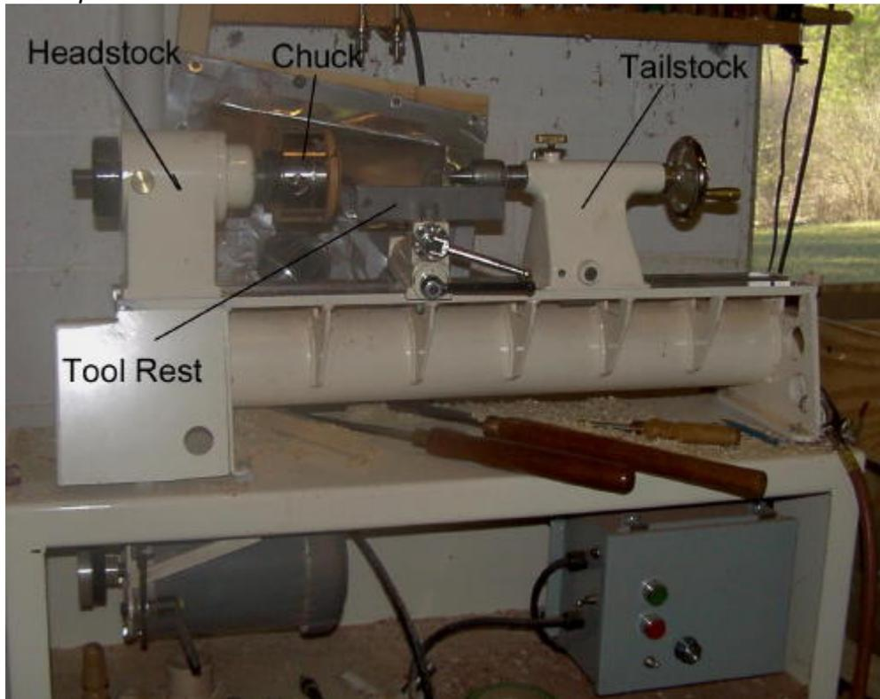
Since the whorls are only roughly circular in shape (and are so even with the circle-cutting jig) the first step in turning is to make them perfectly circular and exactly centered on the hole for the shaft. To do this I mount a plain disk on the lathe, and hold the whorl up against it with the tailstock pressure through the hole in the whorl. The tailstock is centered exactly to the rotation of the lathe, and the cone mounted on the tailstock centers itself in the drilled hole in the whorl.
