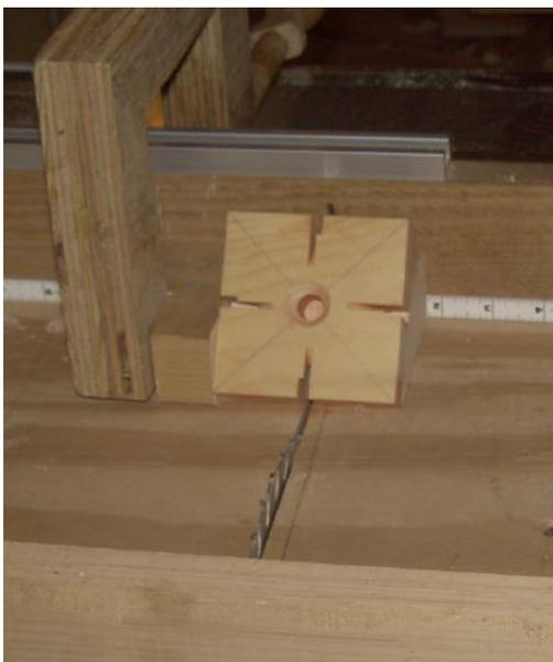
This is my new notch cutting jig, which uses the table saw. Susan wanted to have four notches, so the spinner could use a notch in front, in back, or directly to the side of the hook. Four notches have to be spaced more accurately to look right so I made a carrier the spindle can be attached to (with masking tape so far) as well as a block that tilts the spindle.
