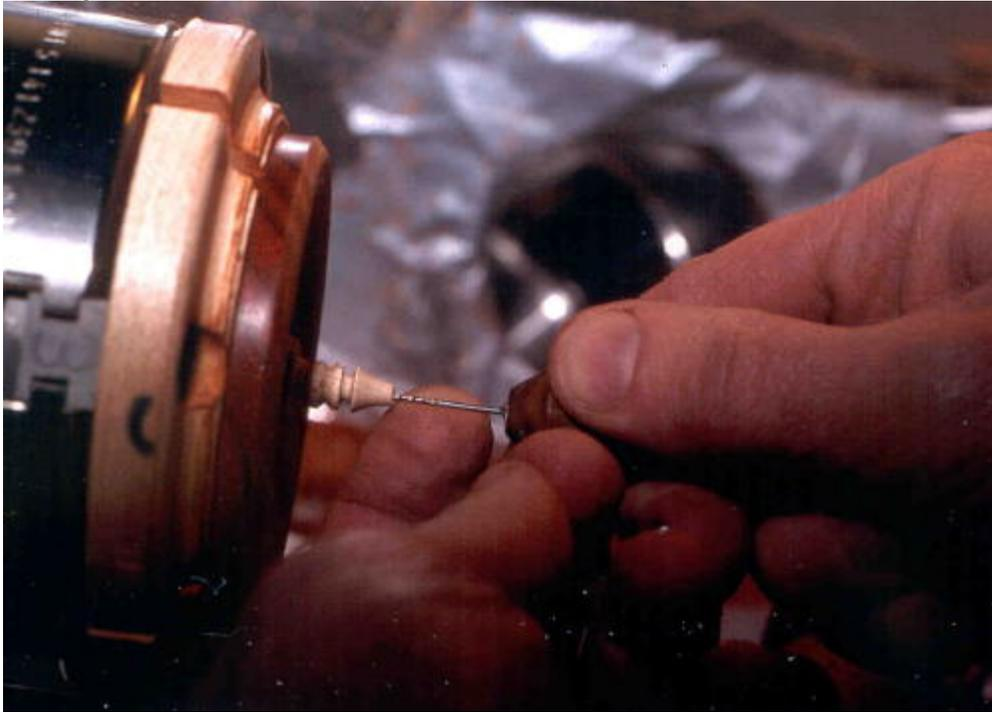
To make the hooks I cut the wire to a length that allows for the depth of the hole and the bends in the hook. Then I use a grinder to round one end of the hook so that it won't be sharp enough to cut fingers. Next I bend the hook to shape with needle nose pliers.
