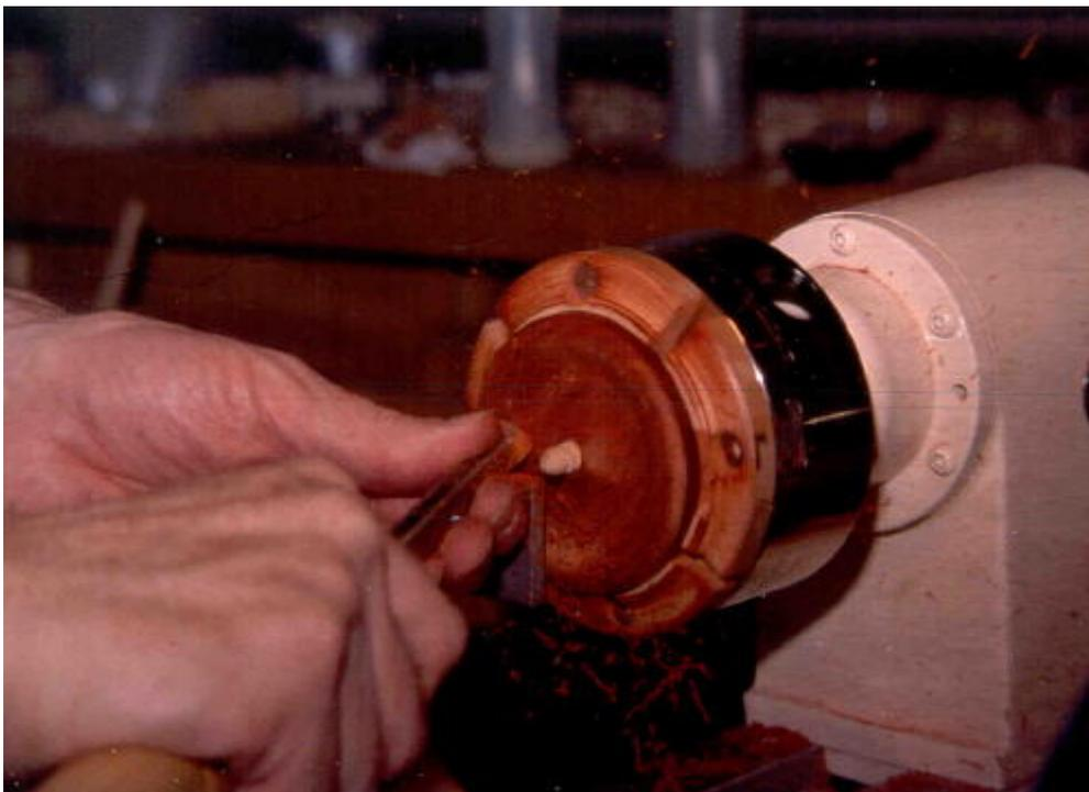
After the whorl is shaped I sand and apply the rubbing finish to the top of the spindle. The last step on the lathe is to drill a hole for the hook. I use a drill bit that matches the size of the stainless steel wire I use for the hooks. The drill bit, mounted in a wooden handle, is pushed into the spinning spindle to create the hole for the hook.
