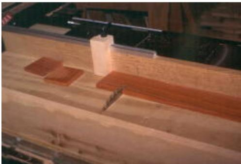
This time I cut the board into squares, then drilled the hole for mounting the shaft on my drill press (a drill press is more or less a hand drill on steroids). By cutting the blank square first, I could use a jig to accurately and quickly locate the hole for drilling
