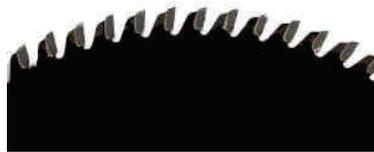
The choice of hook angle is based more on the type of machine used than the material being cut. A blade with a positive hook angle is a faster-feeding blade suitable for a rip cut. A blade with a negative hook angle is less aggressive and suitable for radial arm and miter saws and for cutting metal.
