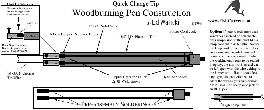
Step 1- Solder pen wires to the power cord jack terminals. Slide wire and jack assembly into the tube to measure wire length. Wires should be cut flush with the end of the phenalic tube, no wire should protrude from the end of the pen tube. Remove the wires and power jack and set aside.
